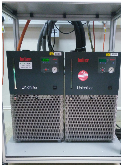
Fig. 5.9 Unichiller device for controlling base temperature
