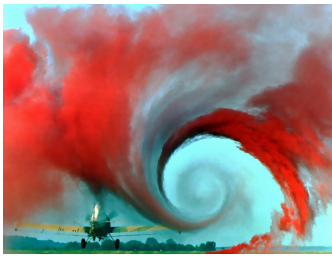
(b) Wingtip vortices behind an aircraft. NASA
